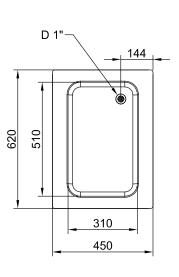
Drop-In Drop-in refrigerated well, static (1 GN container capacity)
